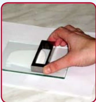
Application on different substrate (glass plate, cement and gypsum boards, wood, metal) – compatibility tests
