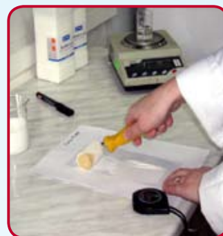
Rolling with an open-pore roller – micro and makrofoam evaluation
